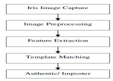
Fig 2 Block Diagram of Stages in Iris Recognition A. Image Acquisition
